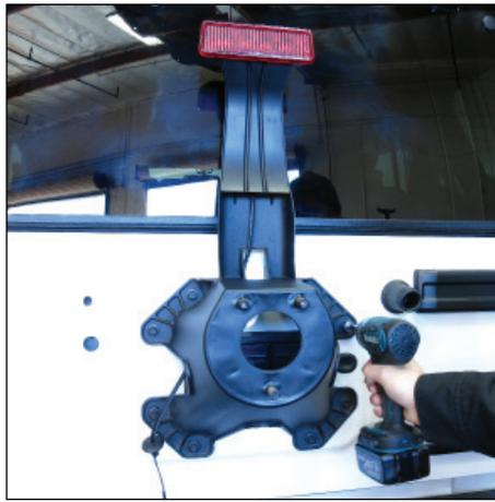
5) Using a 13mm socket, remove all 8 bolts that attach the spare tire mount to the tailgate.
