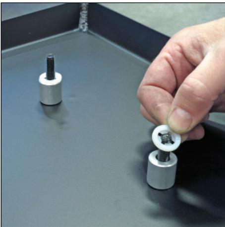
7) Insert the flat head screws from the outside of the panel, and then on the inside, install a spacer and a spacer retainer onto the threads of each screw.
