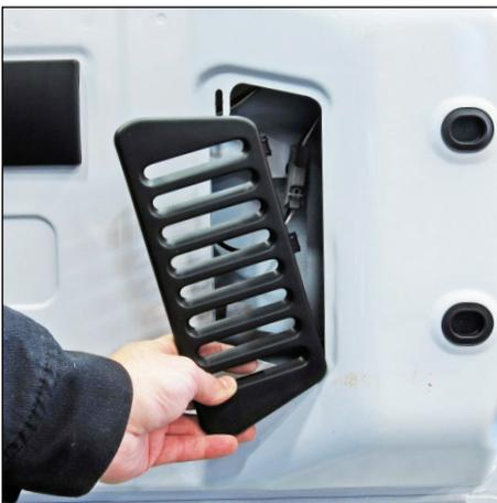
1) Open tailgate and remove access panel with a flat head screwdriver.
