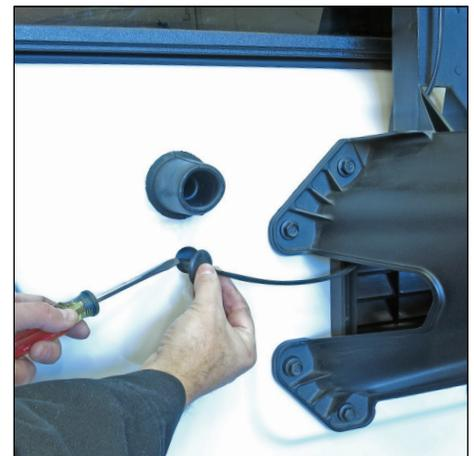
3) Remove wiring harness grommet from the tailgate and pull the wiring out.
