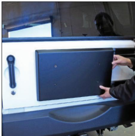
8) Hold the panel up to the tailgate and align the 4 screws. Make sure the vented edge of the panel is facing down.
