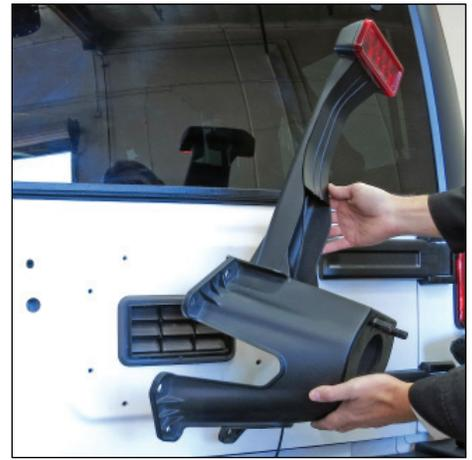
6) Remove the spare tire mount from the vehicle.
