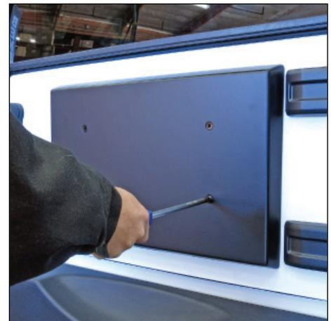
9) Tighten screws with a large phillips screw driver.
