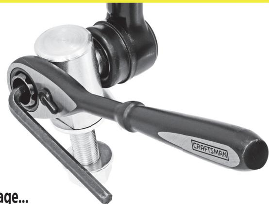
Installation of this kit requires a thru-hole ratchet, shown to the right.
